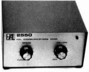
The 2550 features a triggered clock pulse generator, sidetone monitor, iambic keying and dot memory. There's an optional tailormade ID too.
